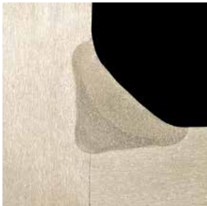
MIG fillet weld in 10mm thick 4140 aluminium alloy using Alulinx gas
