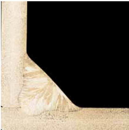
PB MAG (135) fillet in 3mm austenitic stainless steel using Inolinx MAG gas
